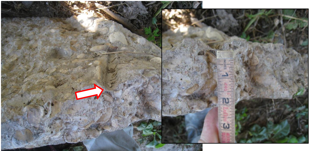
Figure 20. Spall debris from South Bridge Bent 2 spall, exhibiting approximately 2 inches of concrete cover to the reinforcement, based on indentation in debris.
