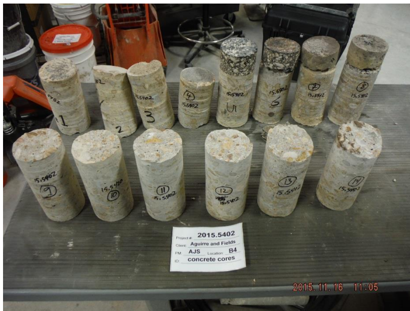
Figure 30. Collection of 14 3-3/4-inch cores obtained from the Austin Avenue Bridges.
