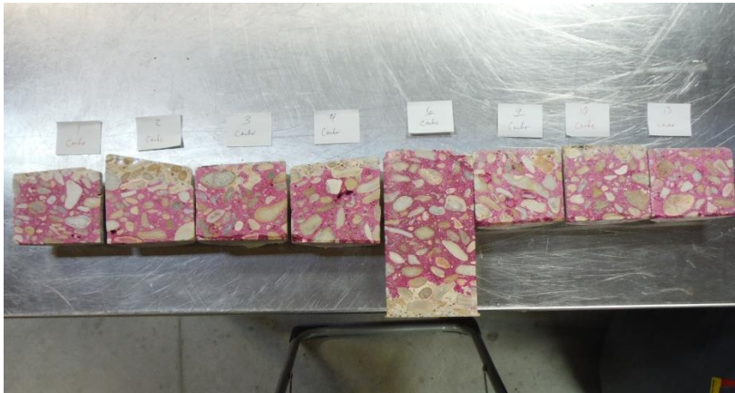
Figure 34. Laboratory investigation of carbonation depth, utilizing phenolphthalein carbonation indicator.
