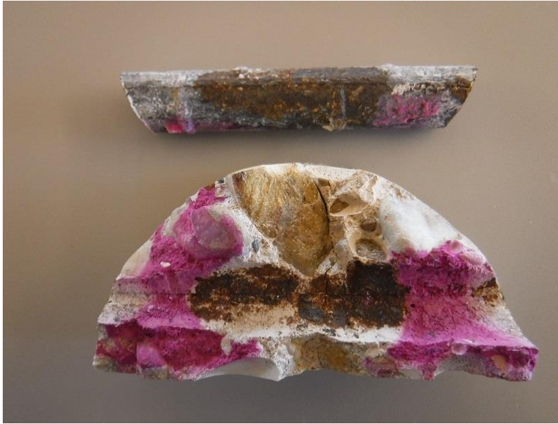
Figure 33. Fractured Core 6, in which reinforcement only exhibits surface corrosion where carbonation depth exceeds concrete cover (non-pink region in middle of core).
