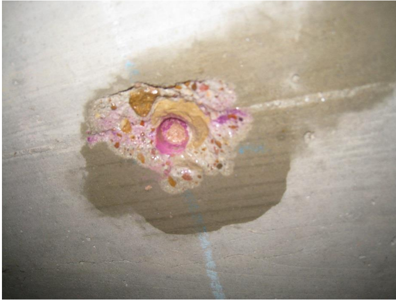
Figure 27. Typical carbonation testing using phenolphthalein solution (pink hue indicates high pH, while lack of color indicates carbonation).
