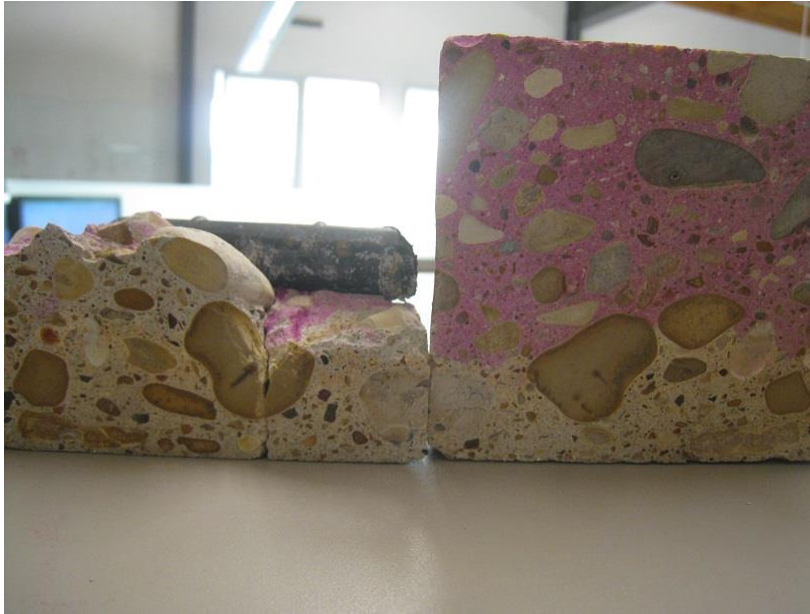
Figure 31. Fractured Core 8, in which the carbonation depth (non-pink region) has not reached the reinforcement, and reinforcement exhibits no corrosion.
