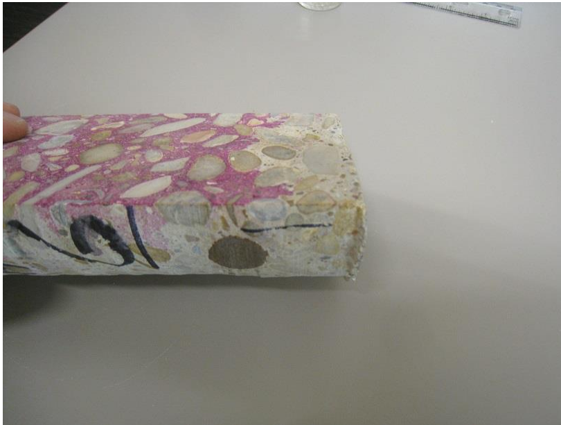
Figure 32. Core 6, with apparent carbonation beyond depth of embedded No. 5 reinforcement.
