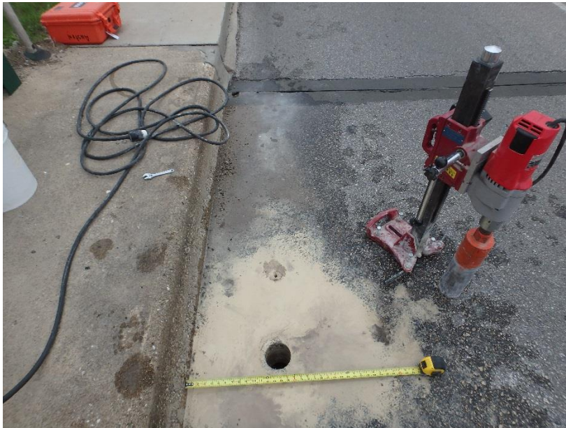
Figure 28. Coring equipment used to obtain 3-3/4-inch cores through Austin Avenue Bridge decks (North Bridge Span 1 shown).
