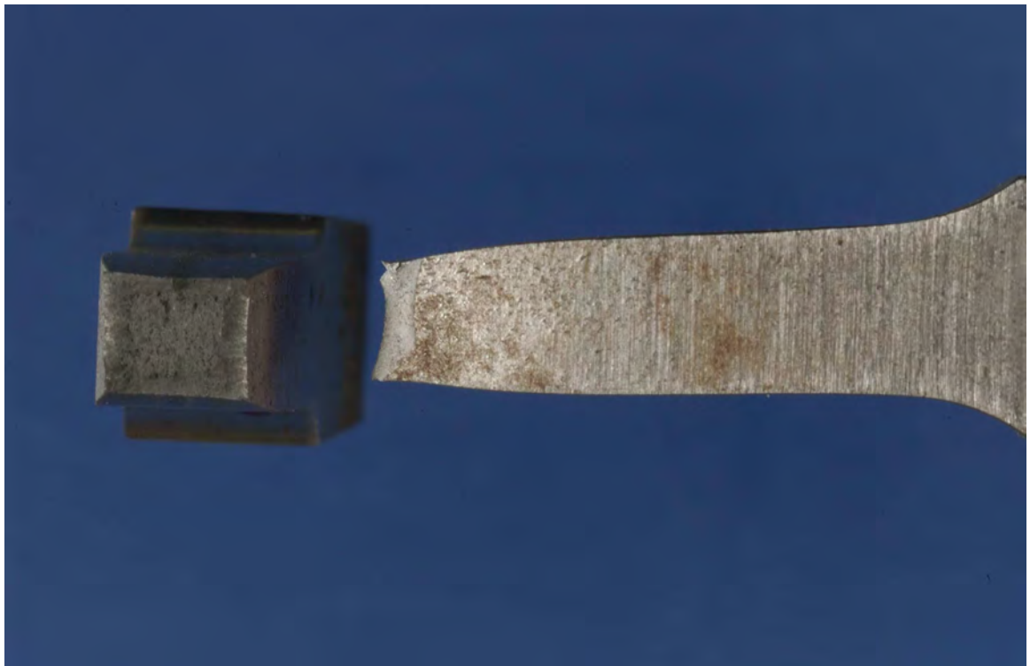
Figure 2. Tensile test specimen fracture on sample N2. L3937 071816 03
