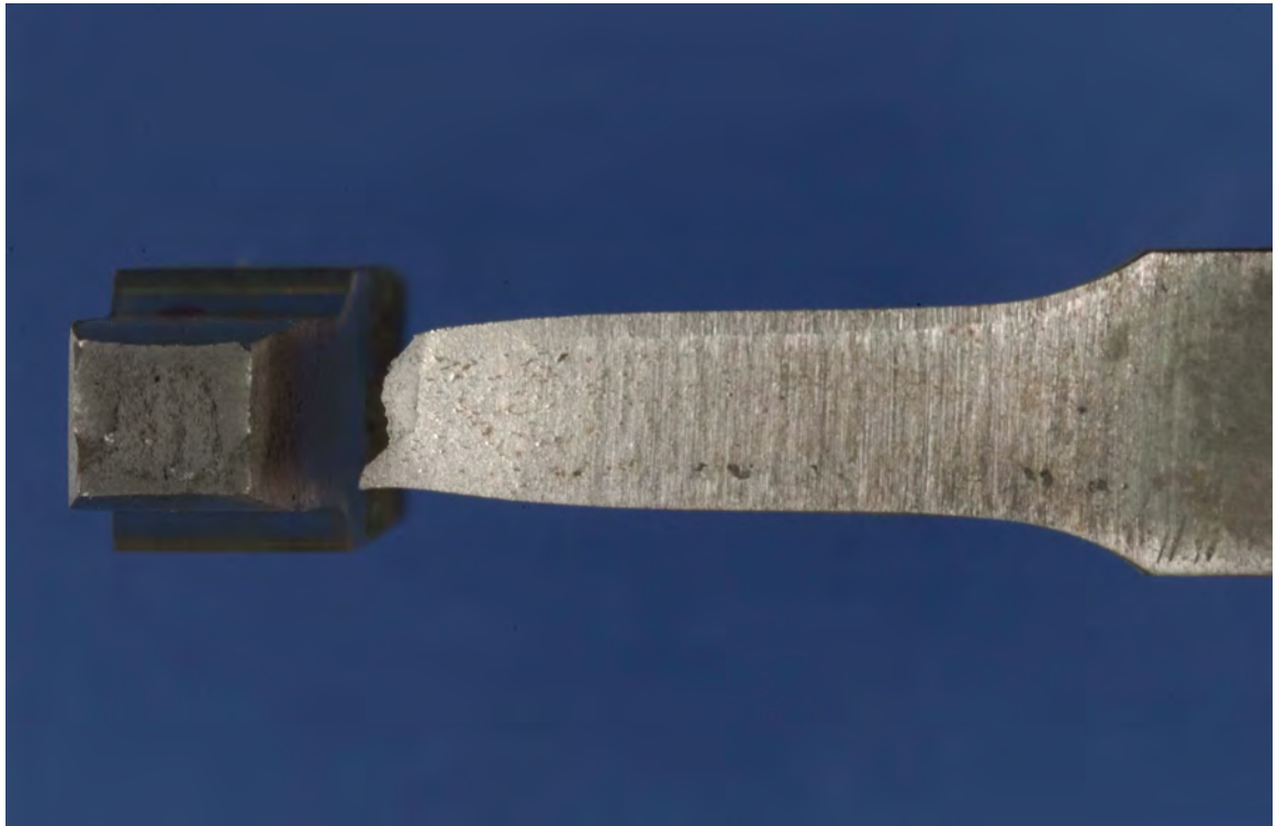
Figure 6. Tensile test specimen fracture on sample S3. L3937 071816 06
