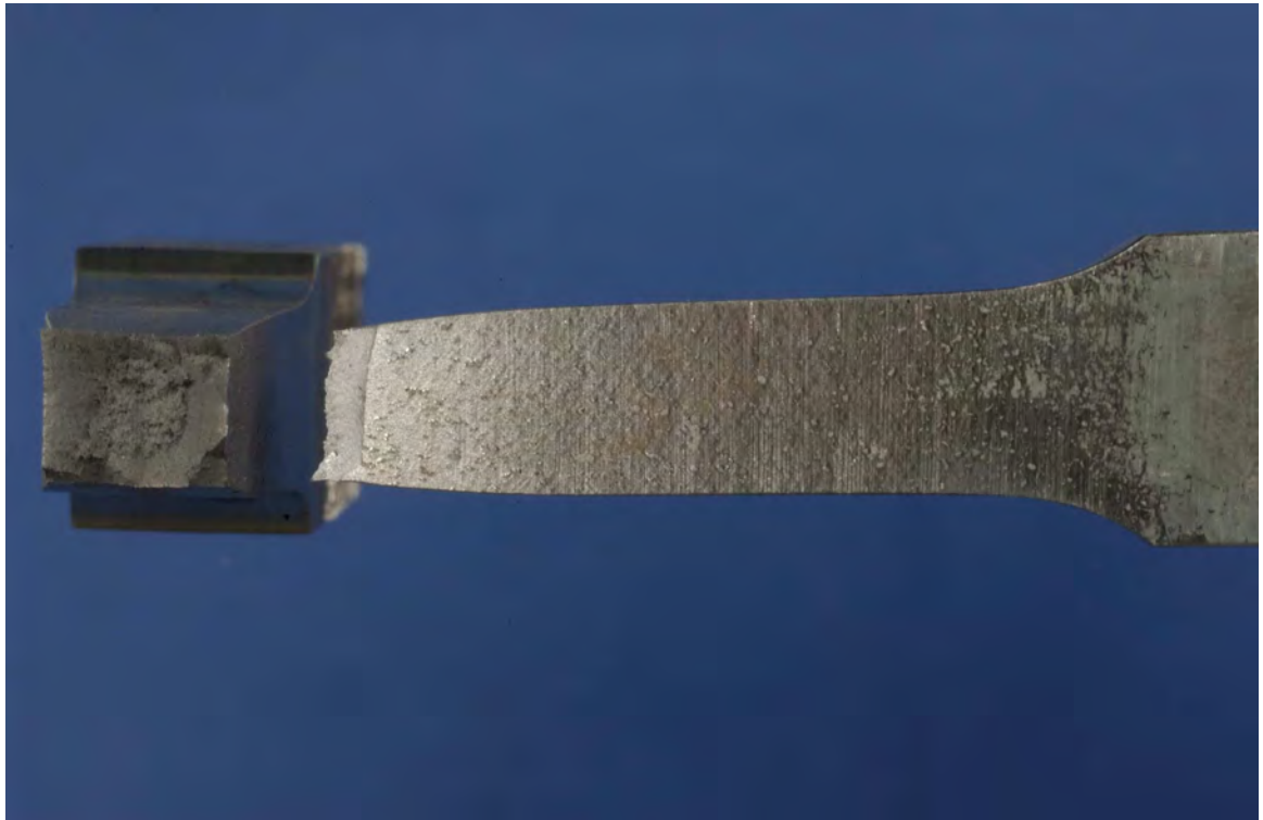
Figure 5. Tensile test specimen fracture on sample S2. L3937 071816 01
