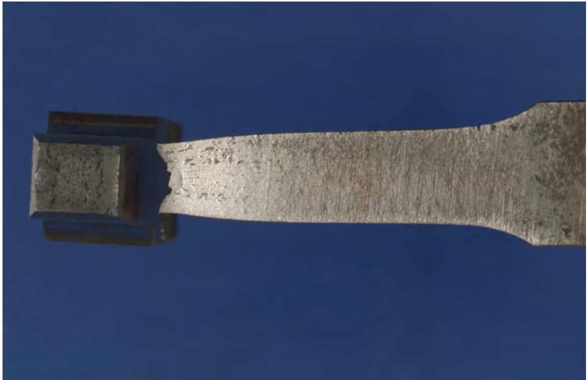
Figure 4. Tensile test specimen fracture on sample S1. L3937 071816 05
