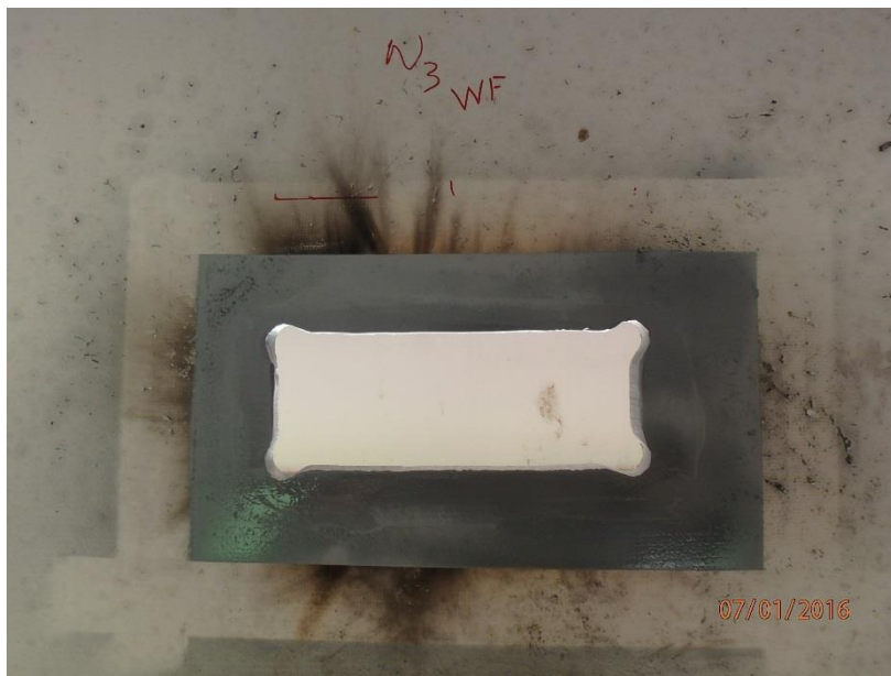
Figure 4. Typical corner grinding and zinc coating application (N3 shown).
