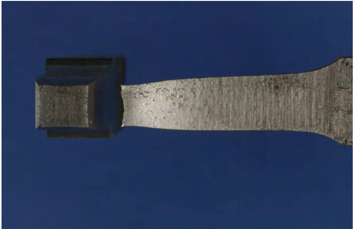
Figure 3. Tensile test specimen fracture on sample N3. L3937 071816 02
