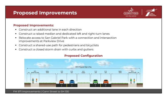
Improvements to FM 971 include constructing an additional lane in each direction, constructing a raised median and dedicated left and right turn lanes, relocating access to San Gabriel Park to the intersection at Parkview Drive, constructing a shared-use path for pedestrians and bicyclists, and constructing curbs and gutters for drainage.
