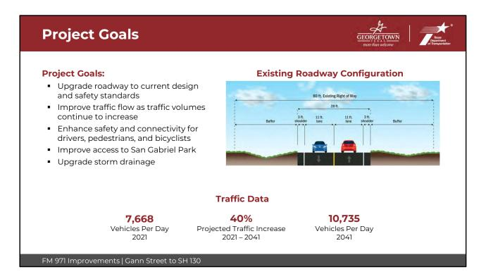
FM 971 is currently one lane in each direction with narrow shoulders, no pedestrian or bicycle facilities, and open storm drainage.
